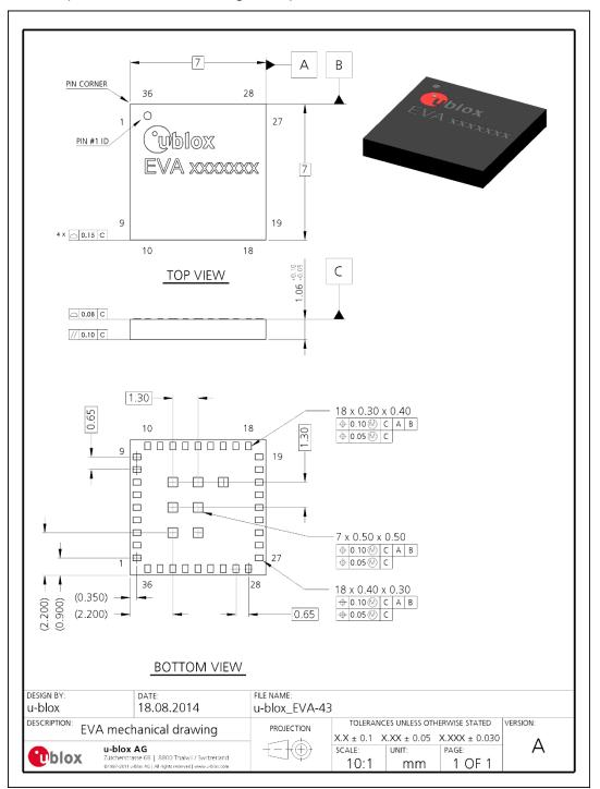
Figure 4: Mechanical drawing for EVA-M8M (LGA43)
