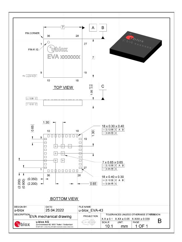
Figure 5: Mechanical drawing for EVA-M8Q (LGA43)
