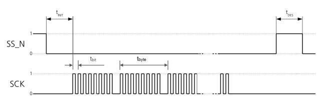
Figure 3: SPI timing diagram
