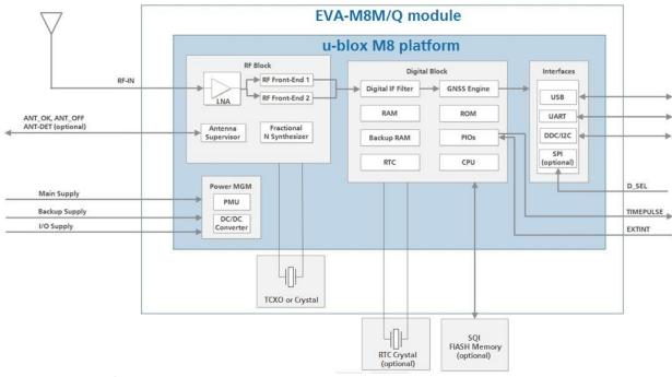
Figure 1: EVA-M8M/Q block diagram
