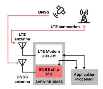
Hardware architecture used in the u-blox SARA-R510M8S combo module.
