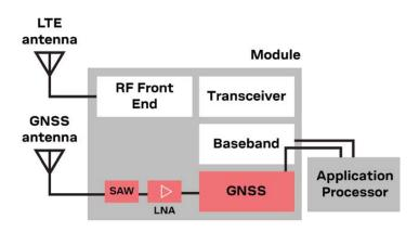
Architectural differences between stand-alone, system-on-chip, and combo IoT tracking solutions.
