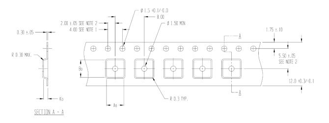
1. 10 SPROCKET HOLE PITCH CUMULATIVE TOLERANCE ±0.2
