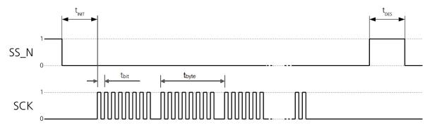
Figure 3: SPI timing diagram
