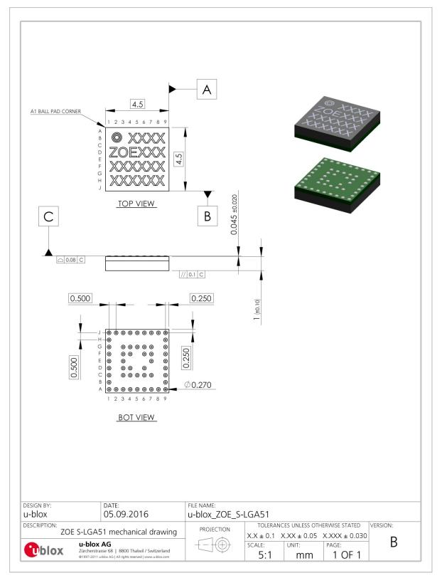
Figure 4: Mechanical drawing for ZOE-M8B (S-LGA), bottom view
