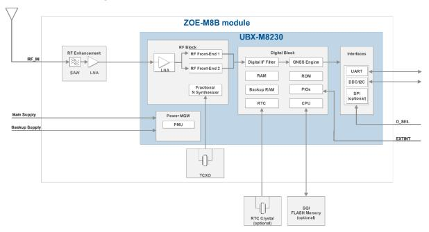
Figure 1: ZOE-M8B block diagram
