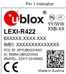
Figure 6: Illustrative example of LEXI-R422 modules' label
