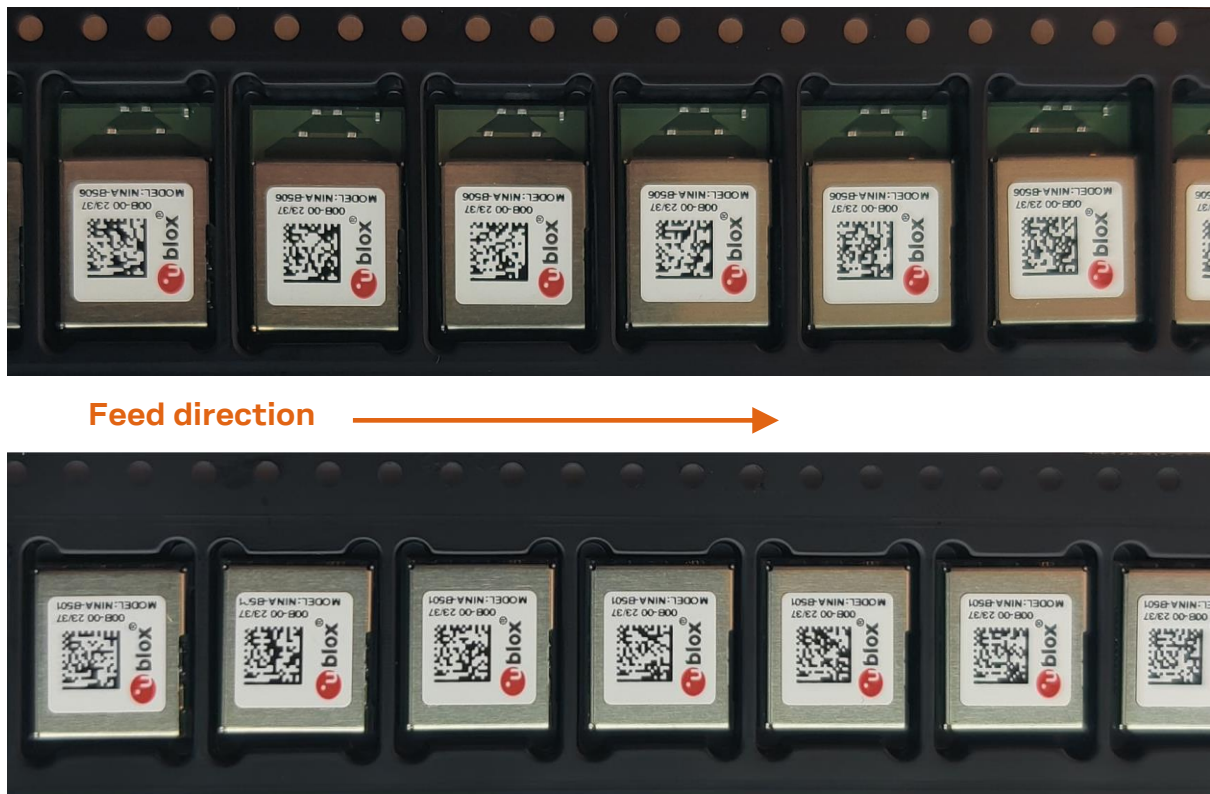
Figure 10: Orientation of NINA-B50 modules on tape
