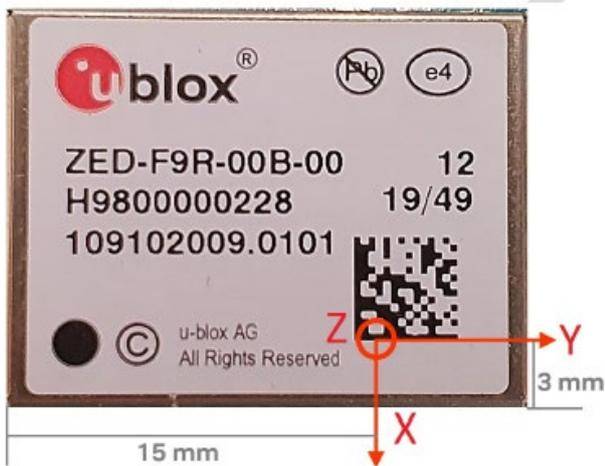
Figure 7: Orientation information. Z-axis points upwards.
