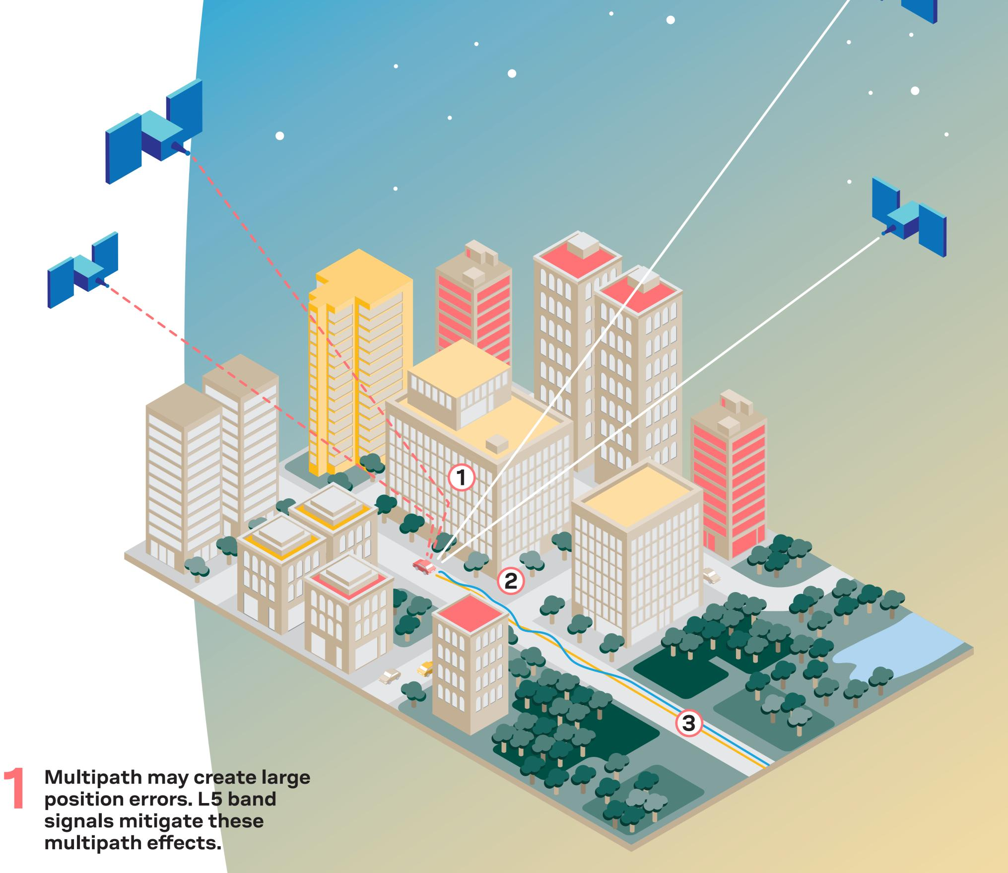
A dual-band receiver in an urban environment is much more accurate than a single-band receiver.
