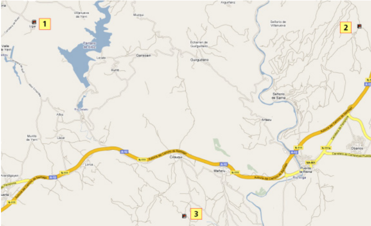
Figure 25: Raster map with three calibration points 6
