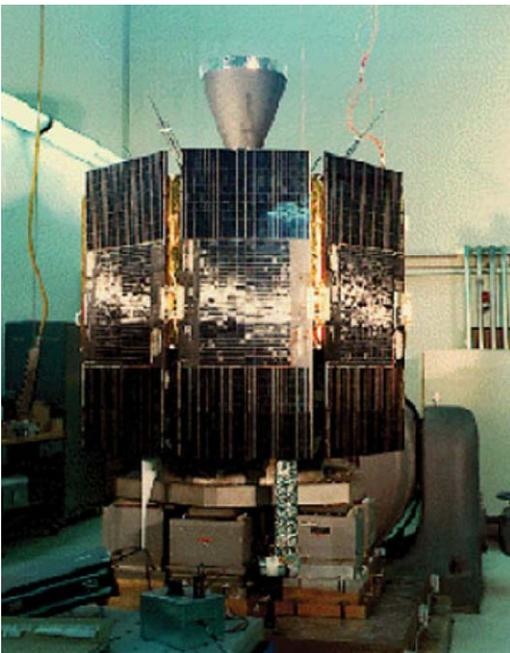
Timation NTS-1 carried two slightly modified commercial rubidium clocks. Unfortunately, attitude-stabilization problems induced temperature variations that masked any quantitative performance evaluation. The atomic clocks were not useful as prototypes for GPS.
