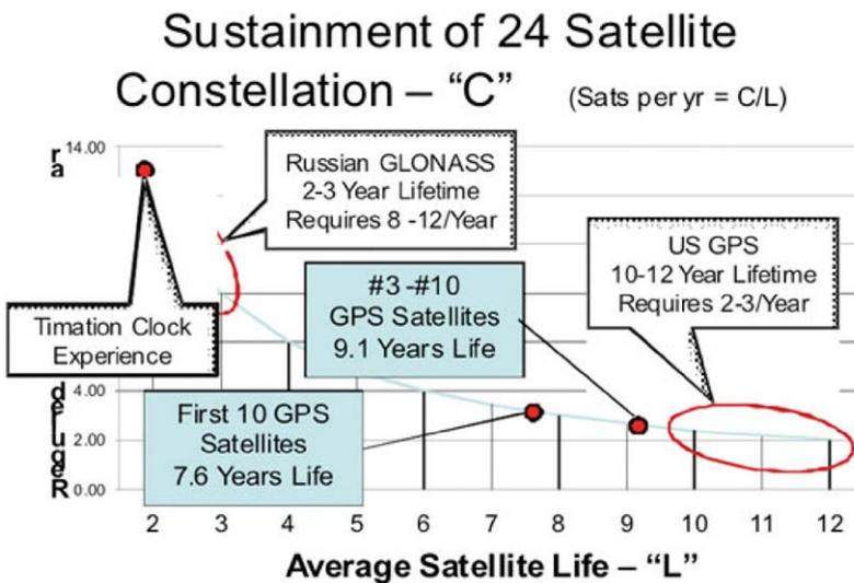
Figure 5. The imperative for long satellite lifetimes.
