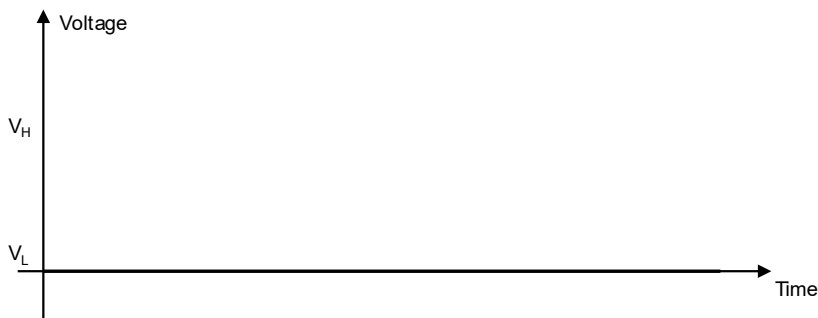
Figure 4: GPIO pin progress for no service
