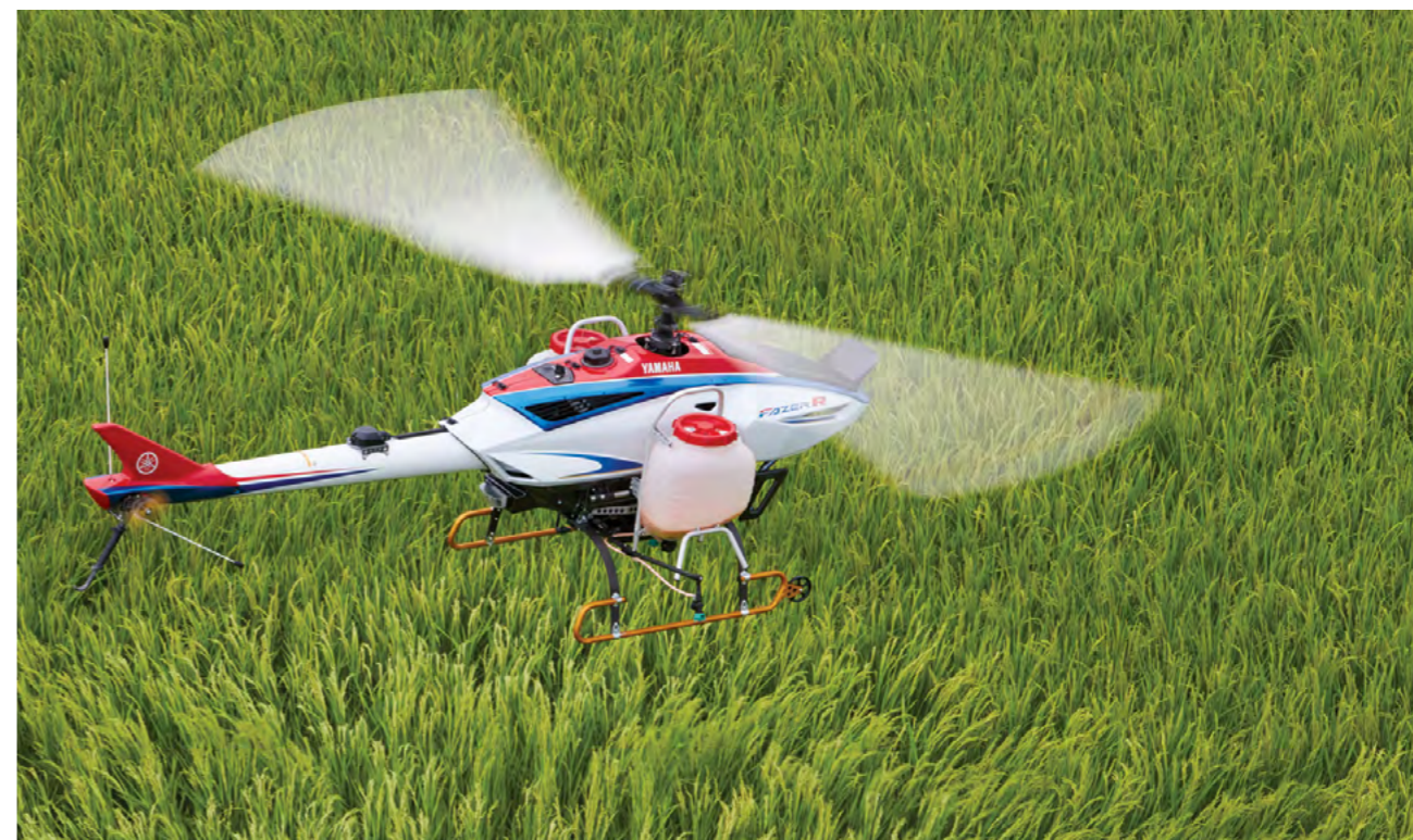
Yamaha Motor's pioneering unmanned agricultural helicopters have long been used to spray rice paddies in Japan.
