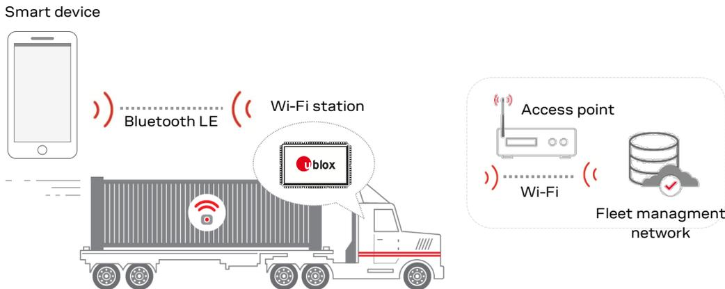
**Figure 33: Example of a u-blox short range module using wireless device configuration**
